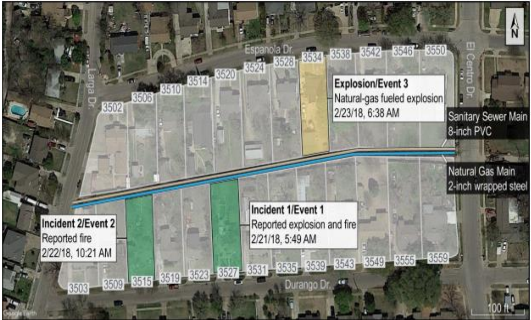
Figure 1. Location of explosion, preceding incidents, and shared utilities.
