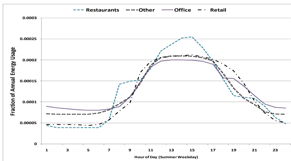
Figure 3-63-6: Load shapes for hot water in four commercial building types
