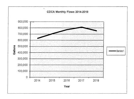
Subsequent to the acceptance of Upper Providence Township as a member municipality of the CDCA, construction of several sewer extensions will significantly increase the number of connections to the system. Based on the current schedule, average monthly flows into the CDCA over the next five years are projected to increase as follows:
