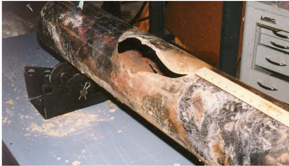
Figure 5. Pipe section containing 12.5-inch rupture
