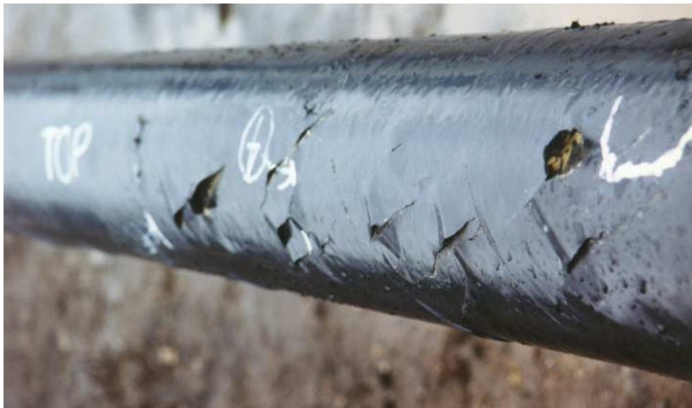
Figure 8. Cracks in the tape coating on 8-inch pipe excavated at accident site
