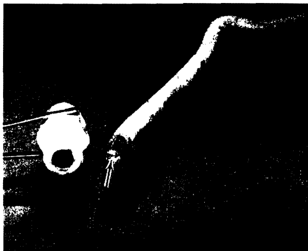
Figure 5: Closer view of tubing and fitting indicated by arrow A in figure 4. Arrow indicates material in end of tubing. The fitting is held by tweezers. X0.54
