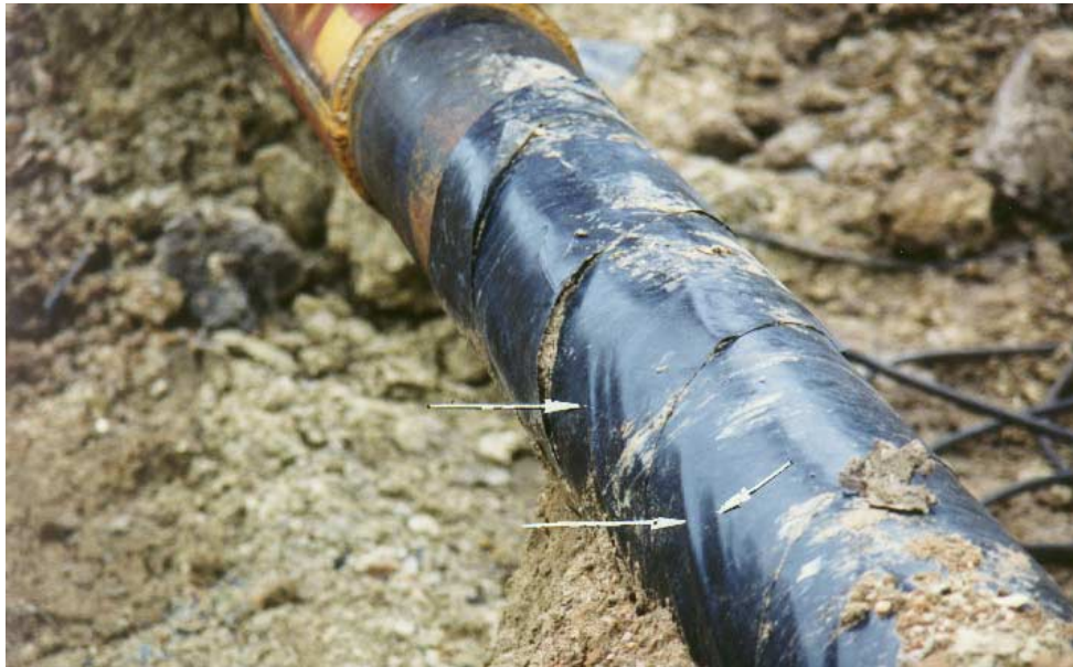
Figure 7. Disbonded tape coating on 8-inch pipe extracted at accident site (Arrows show disbonded area under tape coating.)
