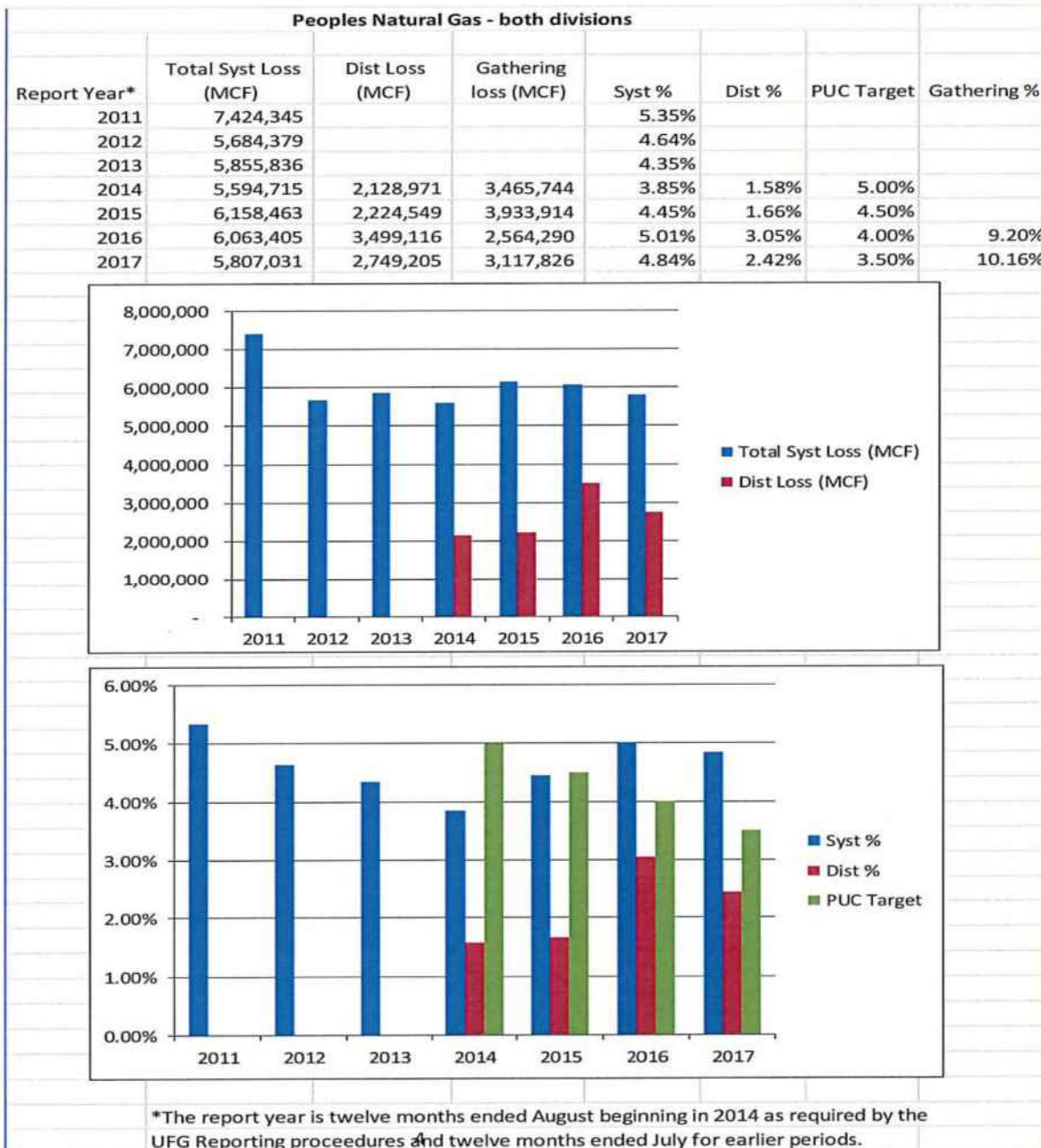
Figure 1: Peoples’ distribution and gathering system UFG reporting (Reference: PNG Exh. No. 2 at 4).
