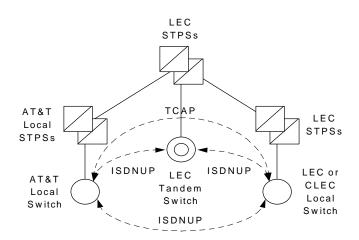
Figure 4. Interswitch TCAP Signaling for SS7 Network Interconnection
