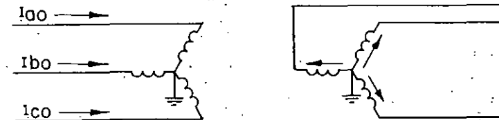
2.22 A circuit connecting with a grounded Y-connected transformer winding with a secondary grounded Y winding on the same core structure.
