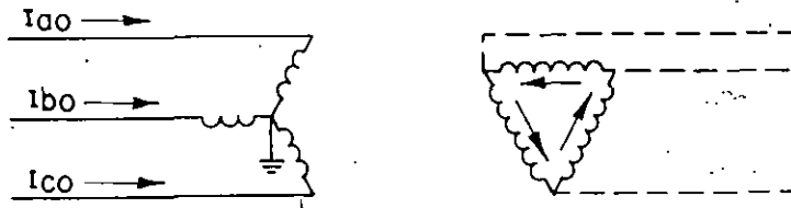
2.21 A circuit connecting with a grounded Y-connected transformer winding with a secondary winding on the same core structure.
