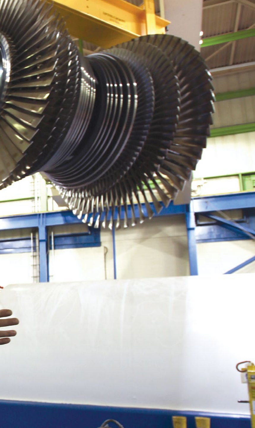
Left: New low-pressure turbine rotors were installed to improve the reliability and efficiency of Unit 1 of our Beaver Valley Power Station in Shippingport, Pa. Below: An Ohio Edison crew member replaces a three-phase power bank as part of a service upgrade for a commercial customer in Akron.
