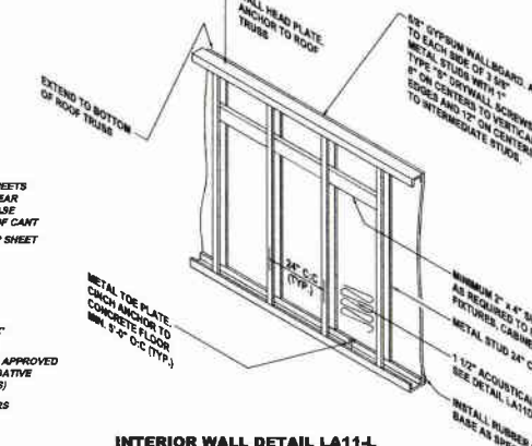
INTERIOR WALL DETAIL LA11-L NOT TO SCALE
