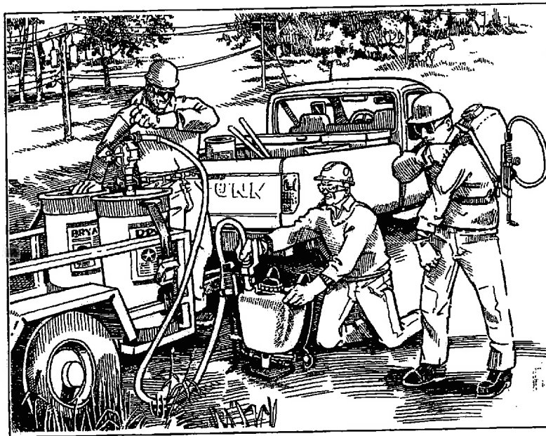
Figure 9. An interlocking valve connection between fill hose and backpack is preferred.
