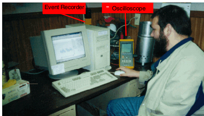
Fig. 1. Electrical instruments used to record power quality data. The event recorder is plugged into a 120-V outlet in the office and the oscilloscope is connected by twisted, shielded cable to metal plates grouted into the floor of milking stalls.
