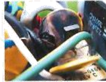
A 130 volt, 150 J MOV that has undergone catastrophic failure, apparently as a result of a lightning strike, showing evidence of heat and smoke. The 3 amp fast-blow fuse immediately in front of the varistor blew during the same event.
