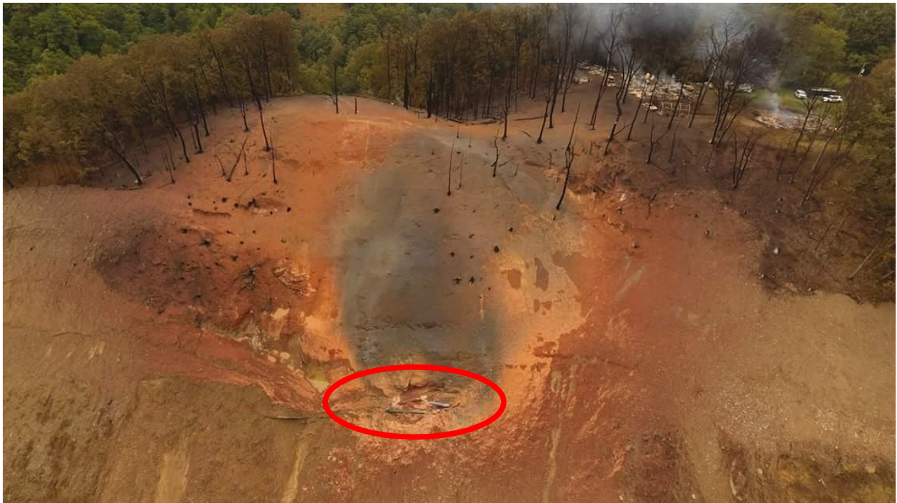
09-10-18 The explosion site the day of the incident. The separated pipe is circled. The destroyed house and garage are smoldering in the upper right corner.
