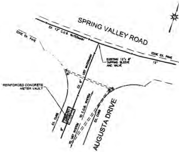
METER VAULT LOCATION PLAN SCALE: 1" = 30'
