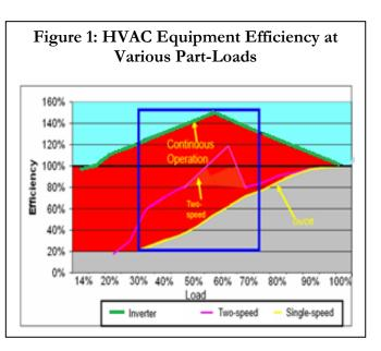
while for single-speed equipment it would yield only a 25% reduction in power consumption<sup>2</sup>.
