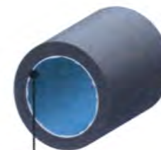
A protective layer of Orthophosphate forms to prevent pipe corrosion.
