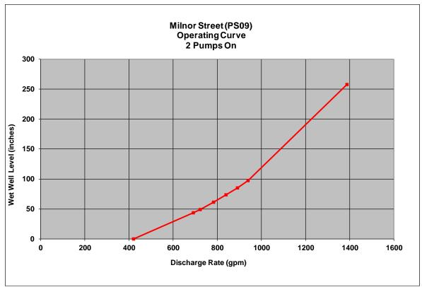
Figure A.7.2.3.3 Milnor Street Pump Station Operating Curve with Two Pumps On
