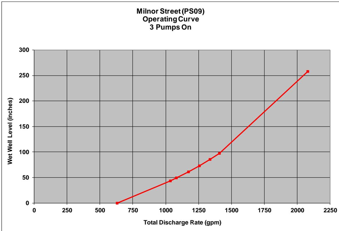
Figure A.7.2.3.4 Milnor Street Pump Station Operating Curve with Three Pumps On
