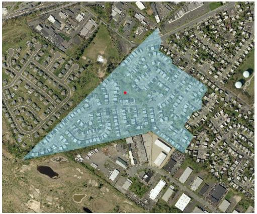
Figure A.7.2.2.1 Contributing Area for the Lockart Street Pump Station
