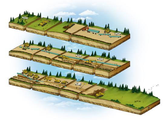
Where workspace and enough land access are available, open trench installation is the typical method used for construction, repair and replacement of various utilities, such as pipelines and sewer and water lines. Open trench installation excavation consists of: digging a trench with backhoes or wheel ditchers; lowering the pipe into the trench; and backfilling the subsoil and separated topsoil, where applicable.
