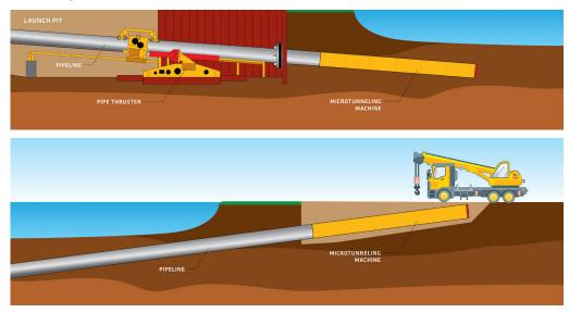
Direct pipe boring is a trenchless technology that combines elements of HDD and tunneling. Direct pipe combines a thruster with a steerable microtunneling machine to install steel pipes in one continuous pass. The direct pipe bore method is effective in all soil conditions, and it uses significantly less bentonite than other trenchless methods, dramatically reducing the possibility of inadvertent fluid returns.
