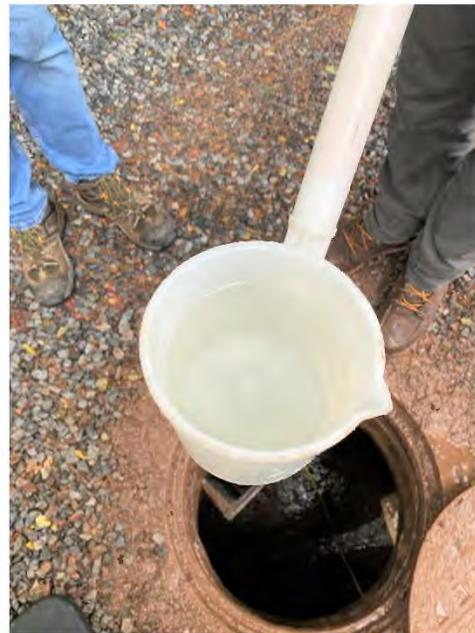
Effluent discharge grab sample 6-27-22 from the ultraviolet disinfection system effluent discharge pipe seen in manhole
