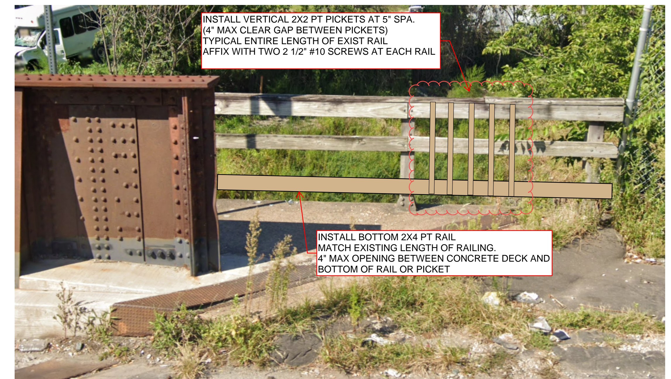
RAILING MODIFICATION DETAIL
