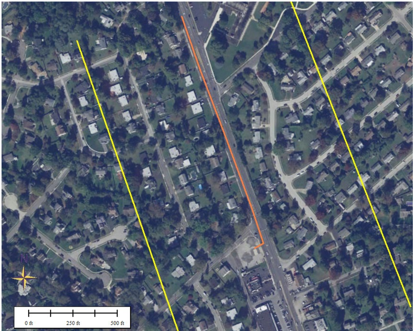
Figure 3. Location of the new 12-inch pipeline in Sproul Road (orange line) in Marple Township south from Russell Elementary School to the site of the proposed transfer station. Yellow lines show the 600-foot limits of “minimum evacuation distance” modeled to meet US Department of Housing and Urban Development recommendations for burn protection (Figure 2) if this line were operated at 475 psig. At 150 psig the limit narrows to 320 feet, on each side of the pipe, still encompassing many homes. This October 2020 airphoto is from GoogleEarth.
