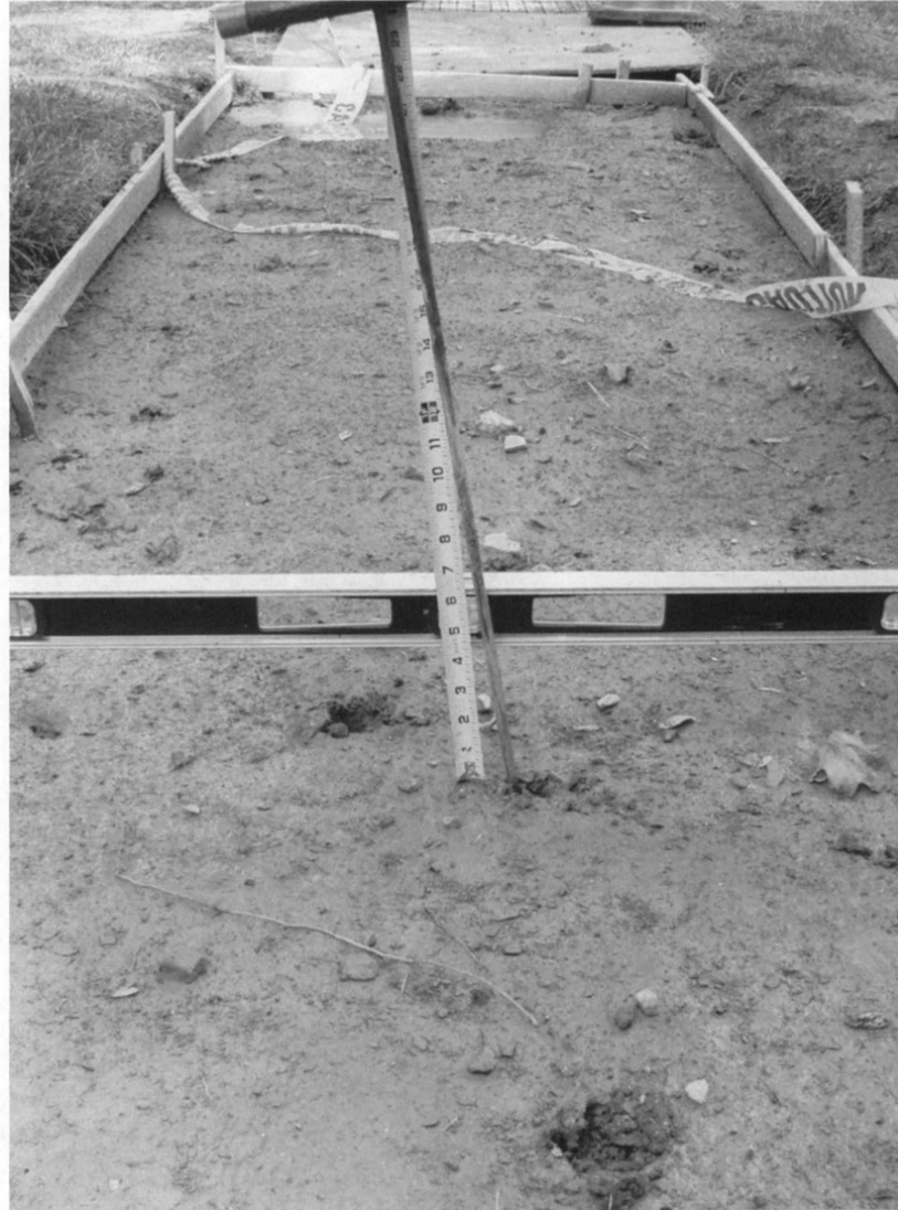
P2 339 PEPPER ROAD - SOIL PROBE DEPTH 24-INCHES BGS LOCATION ID : SLAB CENTER LENGTH - CENTER OF WIDTH DATE/TIME : 20220613_1109AM FOTO ID : P6137585_RS_
