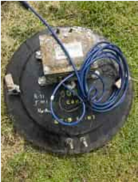
▲ The collection system in South Bend, Indiana, contains approximately 160 sensors, enabling real-time monitoring of flow and level measurements.
