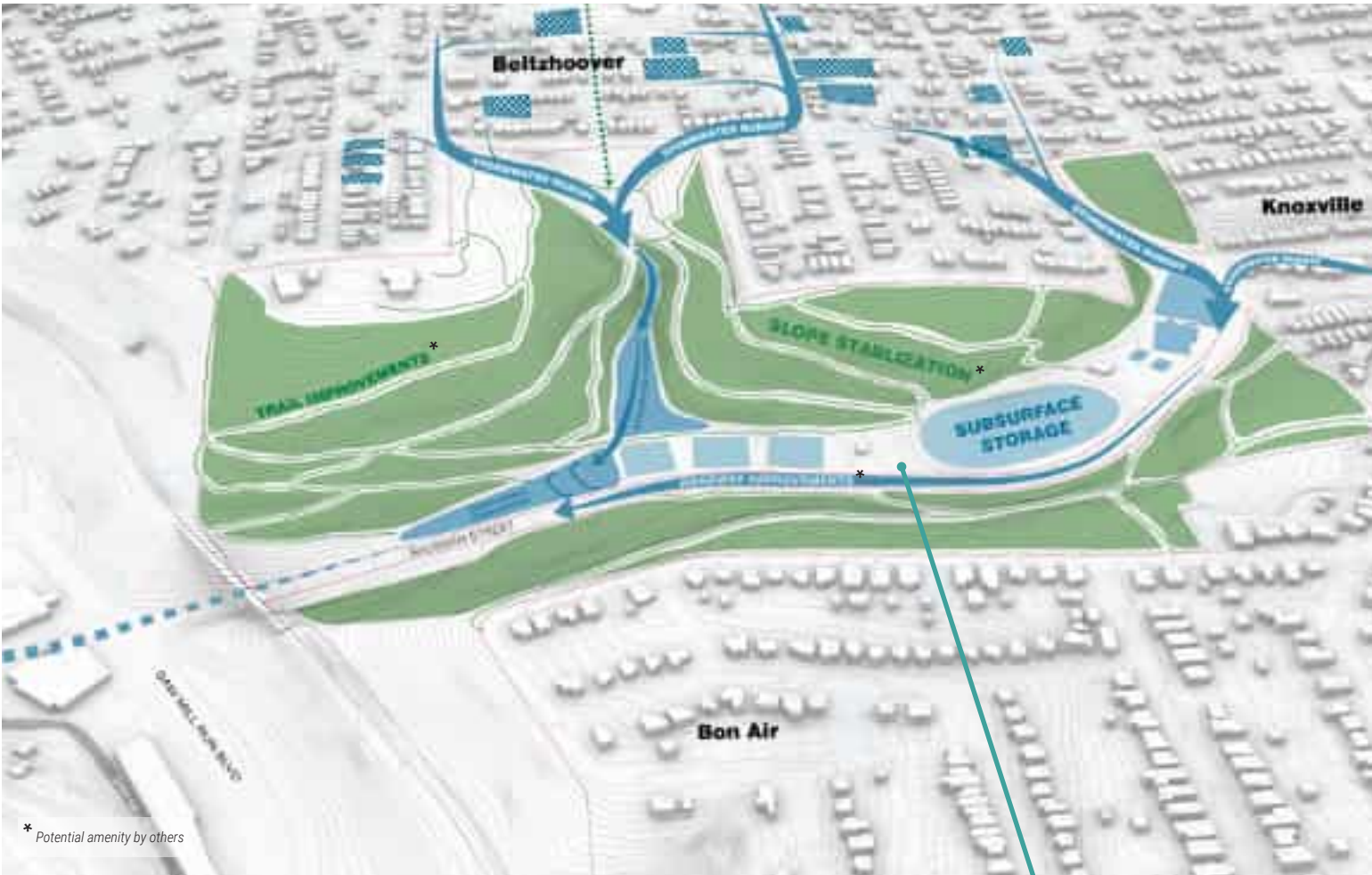
Diagram of the example site, showing potential features and stormwater engineering strategies, including subsurface storage, with additional improvements by others.
