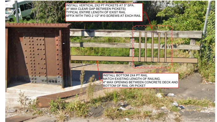
RAILING MODIFICATION DETAIL
