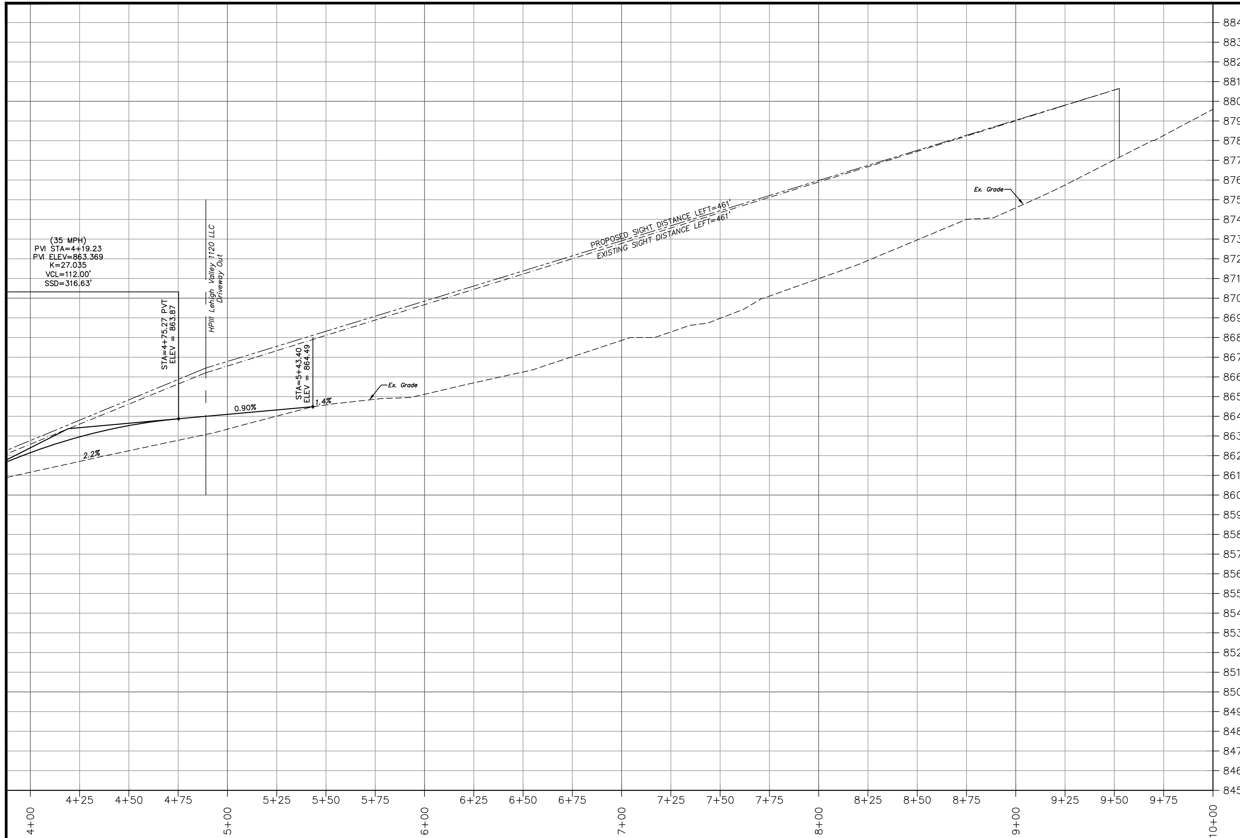
Horizontal Scale : 1" = 25' - Vertical Scale : 1" = 2.5' Profile - OAK STREET CENTER LINE
